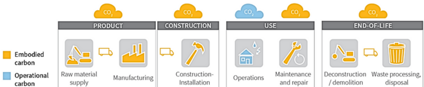
Figure 3: Embodied carbon (yellow) and operational carbon (blue) across the key life cycle stages of a building (Carbon Leadership Forum, 2020)
